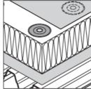
Overlap length between sleeve and fastener: 15mm
