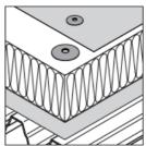
Overlap length between sleeve and fastener: 13mm
