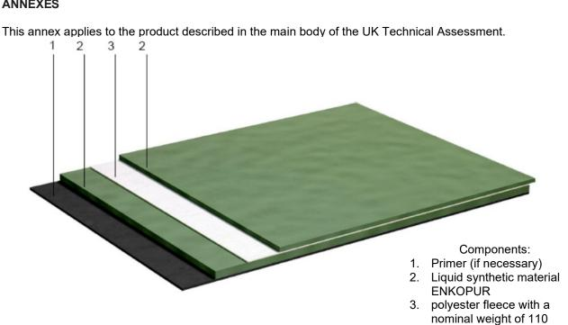
Applicable to the roof waterproofing **ENKOPUR**
