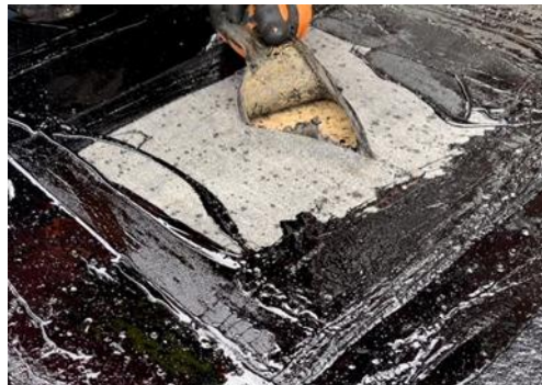
Fig. 5 - MOY Paromelt (Fail) – The MOY Paromelt Compound and Primer have peeled cleanly from the deck, indicating a failure in bond between the primer and the concrete substrate.
