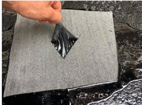
Fig. 4 - MOY Paromelt (Pass) – The MOY Paromelt Compound is displaying strong bond to both the concrete substrate and the MOY Paromelt Protection Layer.
