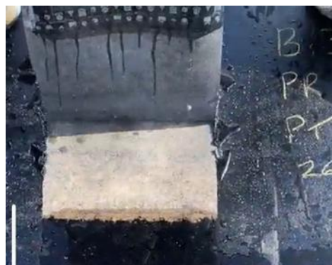
Fig. 2 - Reinforced Bitumen Membrane (Fail) – Membrane and primer have peeled cleanly from the deck, indicating a failure in bond between the primer and concrete substrate.
