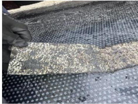
Fig. 3 Reinforced Bitumen Membrane (Fail) – Membrane has peeled easily from the deck with laitance visible on the reverse of the membrane.
