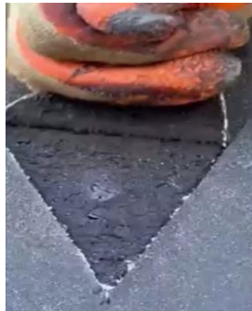
Fig. 1 - Reinforced Bitumen Membrane (Pass) – Membrane is showing a cohesive failure between layers indicating a strong adhesion to the concrete has been achieved.
